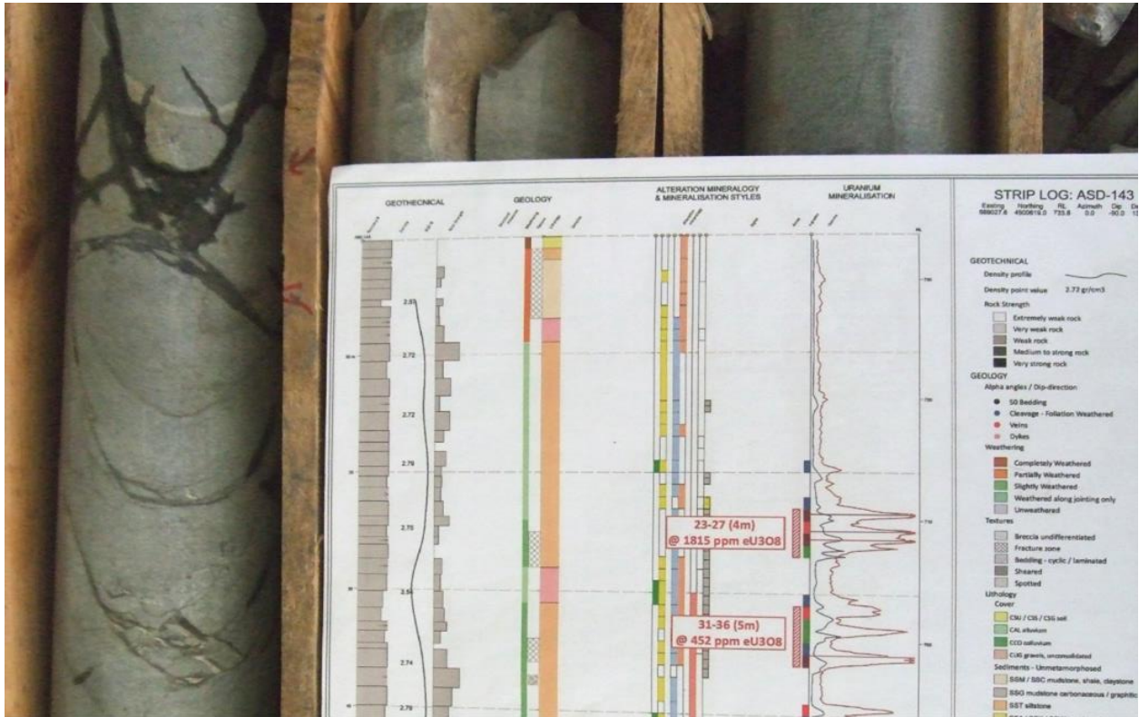
Figure 3-2. Drill core box with late-stage open fractures with pitchblende and typical Berkeley logging sheet
